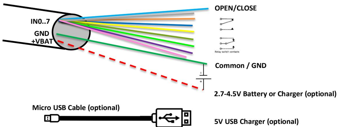
Try to align wiring to below Generic Profile, otherwise custom profile is needed:
